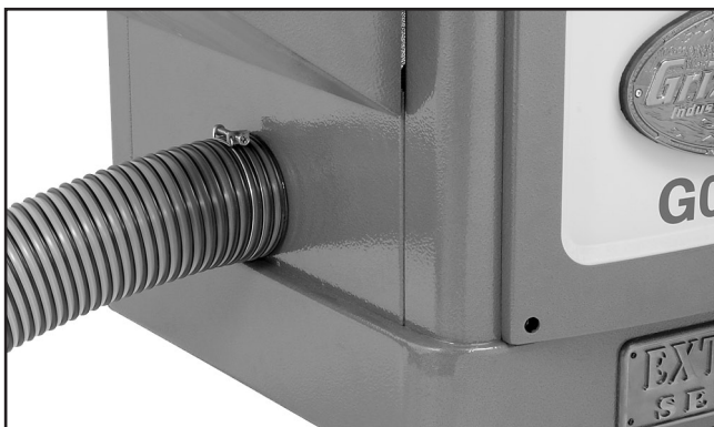
Figure 35. Dust hose attached to dust port.
